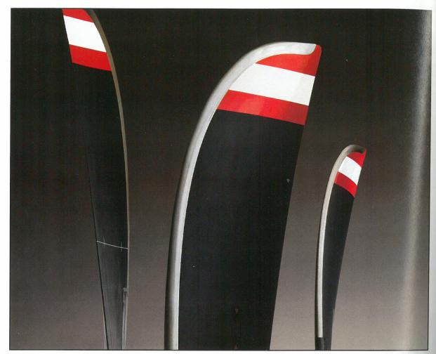
If you're thinking of snickering at the odd-looking propellers on the new C-130J Hercules, think again. Simply by twisting the blades a bit and increasing their number to six, we've given the aircraft 18% greater thrust at the same power setting.
